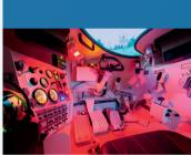
The tank driver training simulator is used for initial and advanced military driver training for the Leopard 2 main battle tank. The system replicates the original driver's station of the vehicle. Operator interfaces, control gauges and observation devices all largely correspond to the original equipment, thus enabling highly realistic training. Vehicle physics is dynamically simulated, considering, among other attributes, the vehicle speed, steering angle and various ground conditions.
